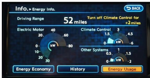
before the car will go into limp-home mode with approximately 2% of available charge remaining. Limp-home mode allows you to travel approximately 1.5 to 2 additional miles (depending on driving style and conditions) at reduced speed. For trip planning, GHD staff use a practical range limit of about 70 miles per full charge. This allows for use of climate control as needed and provides a range buffer for getting to the final destination.
