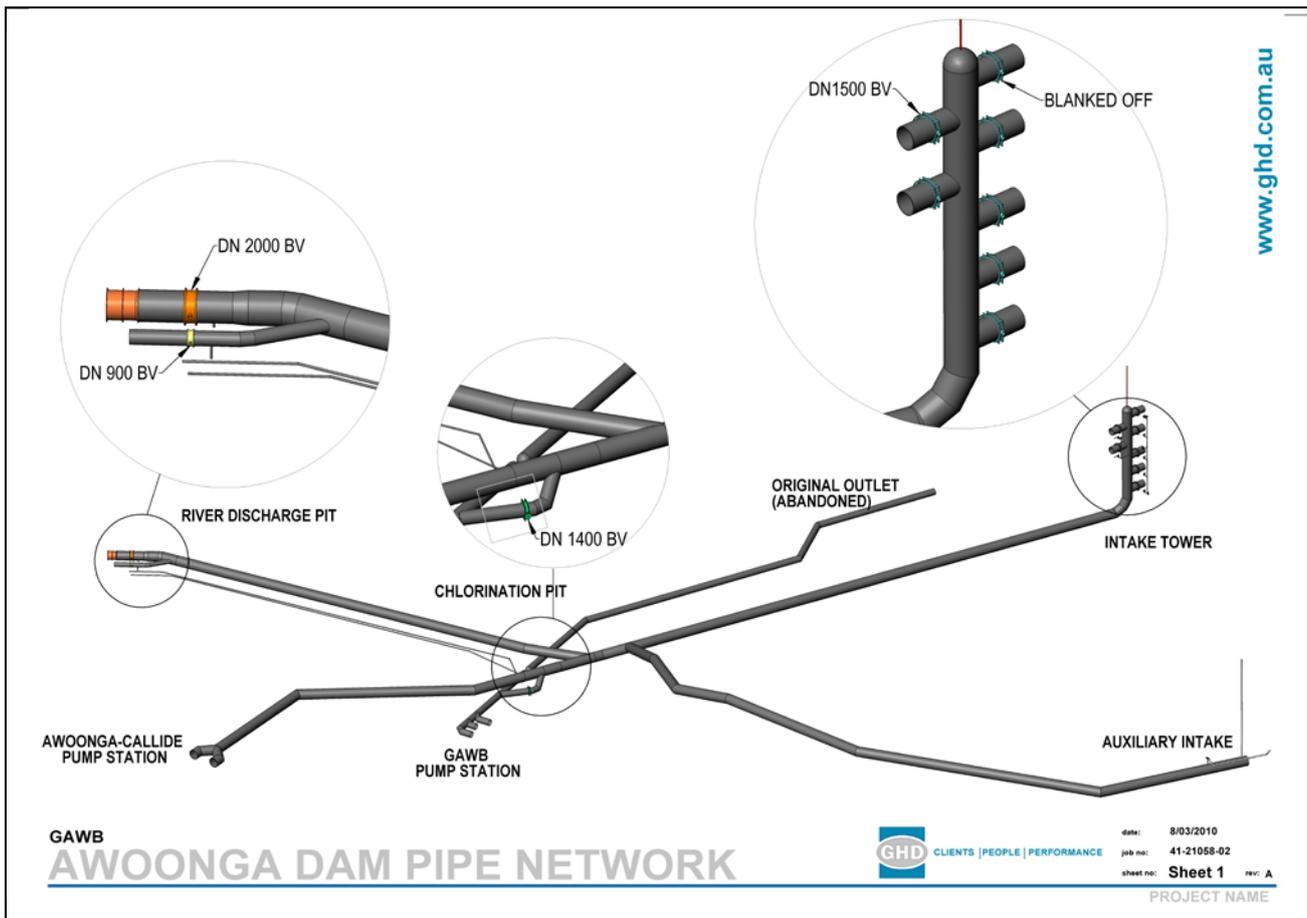
**Figure 1:** Layout of outlet pipe work
