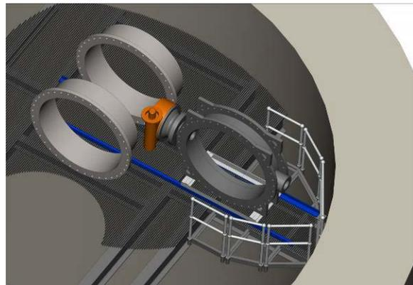
**Figure 5:** 3D simulation of tower valve removal
