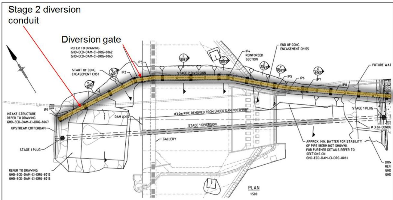
Figure 1: Plan view of diversion conduit.
