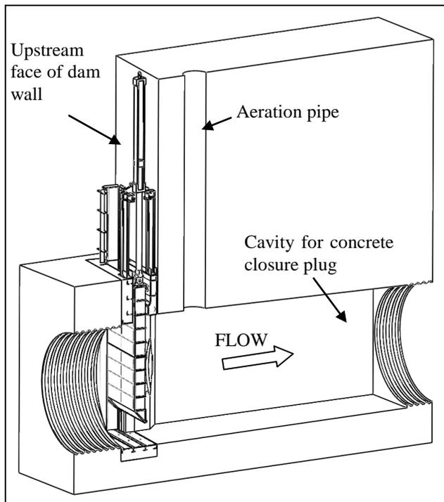
Figure 2: Sectional view of gate in conduit.
