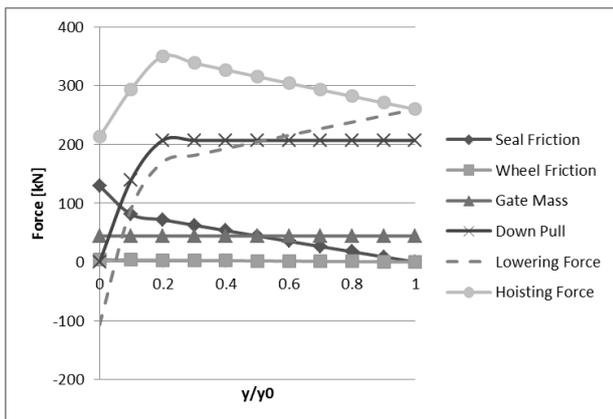
**Figure 5: Forces on Gate at maximum head**
