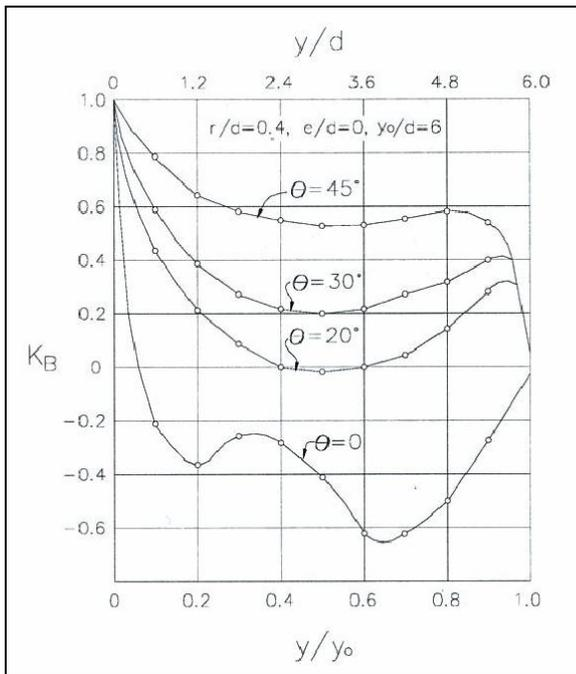
**Figure 4: Variation of  $K_B$  with relative gate opening for various  $\theta$ . *Erbisti*<sup>1</sup>**
