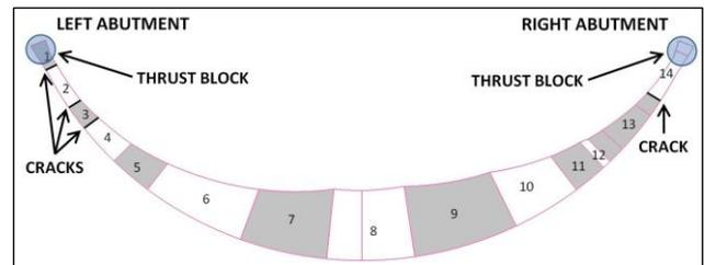
Figure 5: Dam base sections for sliding assessment
