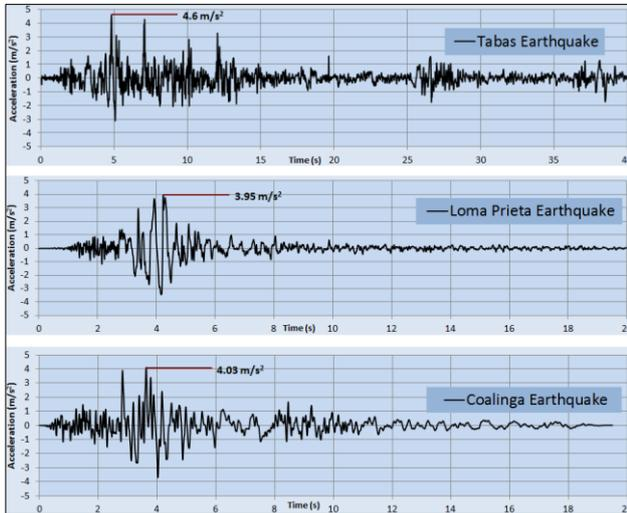
**Figure 2: Acceleration time-histories (only most demanding horizontal component shown)**
