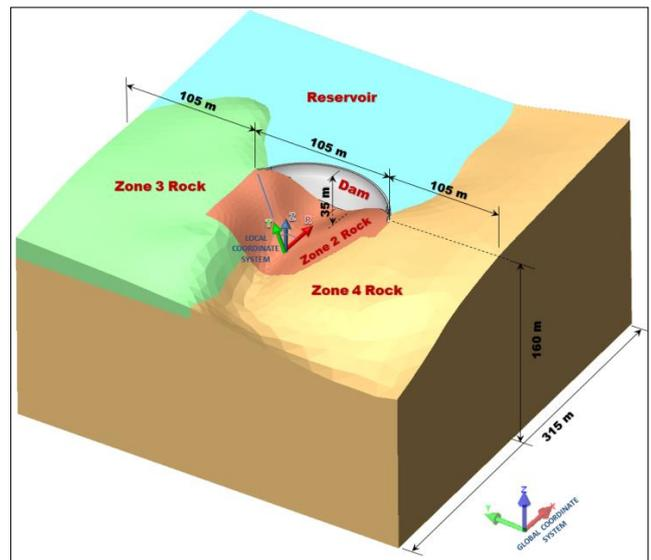
**Figure 3: Rendered FE model of Barossa Dam**
