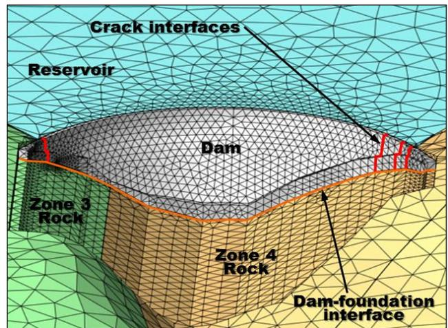
**Figure 4: Nonlinear contacts in FE model**
