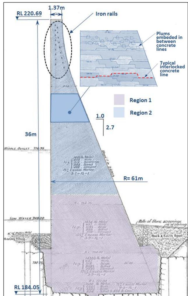
Figure 1: Barossa Dam - Details of maximum section
