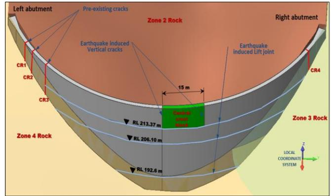
**Figure 9: Expected cracking on dam wall after MDEs**
