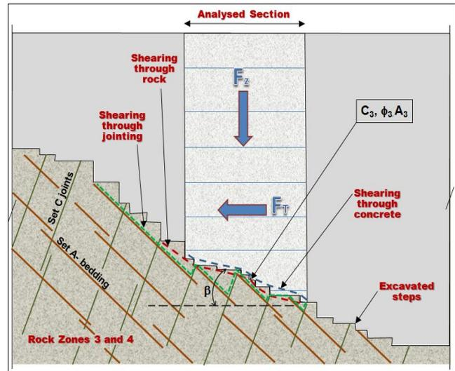
**Figure 7: Arch (tangential) sliding assessment**
