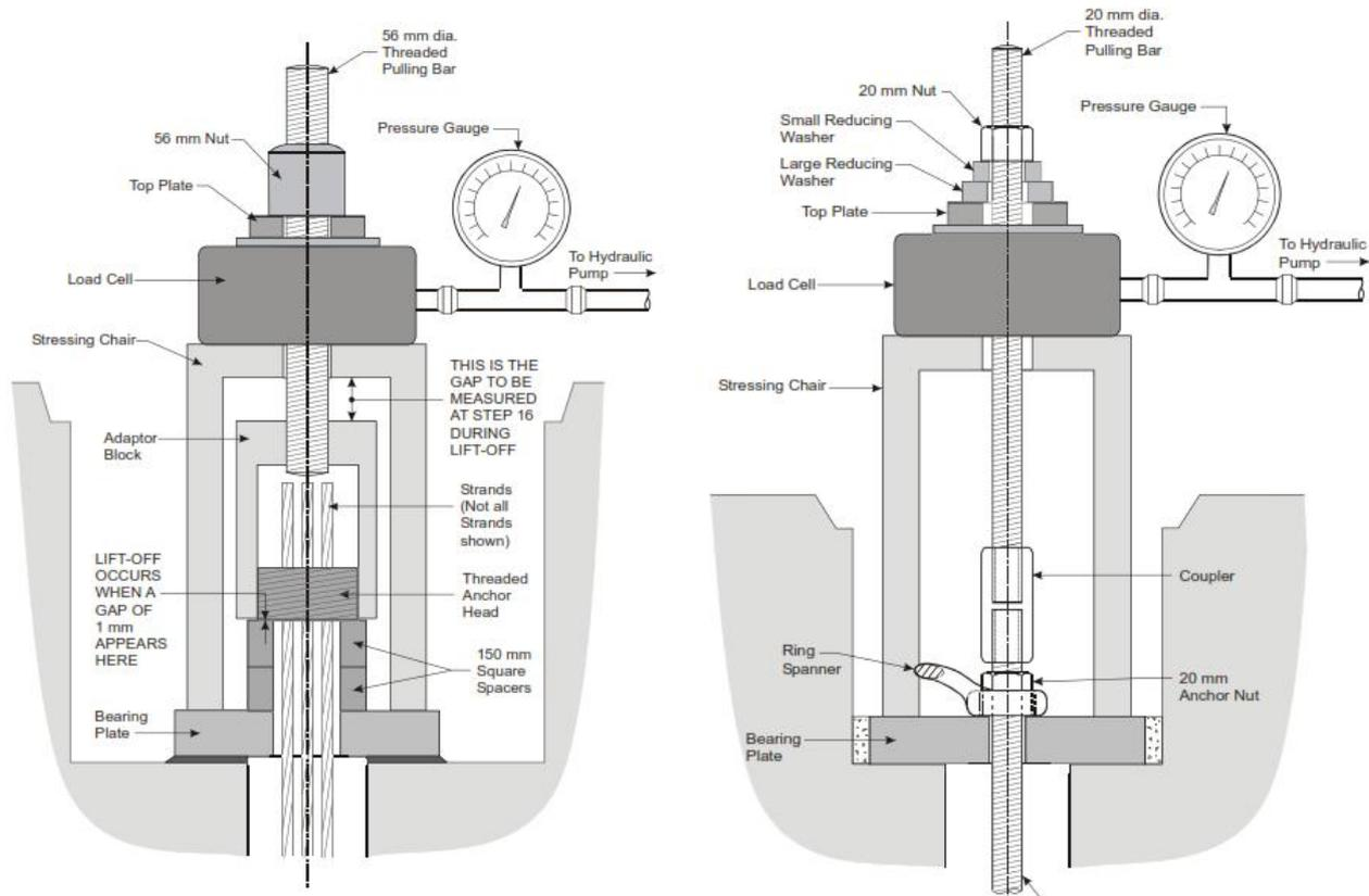
**Figure 1 Example lift-off testing setup for strand anchor (left) and bar anchor (right)**
