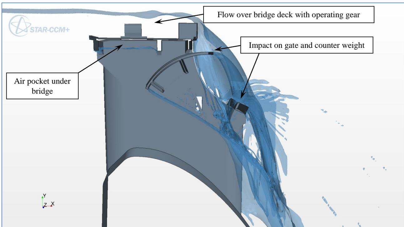
Figure 2: CFD water level results for the existing crest arrangement (115.0 m AHD reservoir water level).
