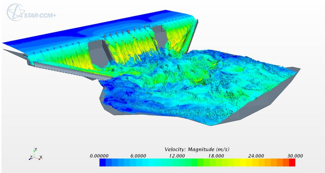
**Figure 4: Surface velocity results for a proposed crest arrangement.**
