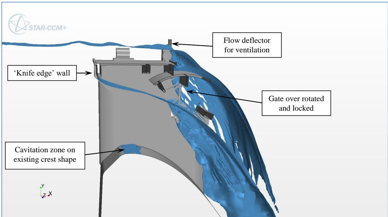
Figure 3: CFD water level results for the modified crest arrangement (115.0 m AHD reservoir water level).
