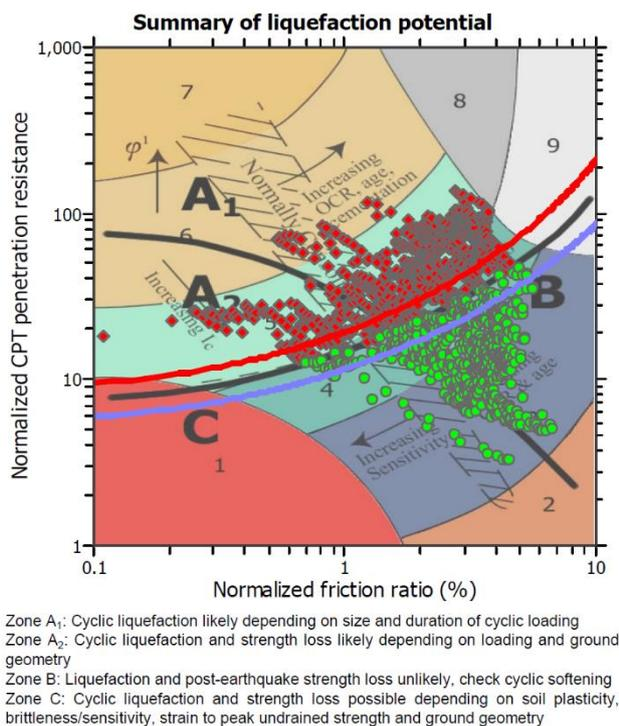
**Figure 5. Results of liquefaction susceptibility for a sample CPT probe at crest of ash embankment in HAP4A**
