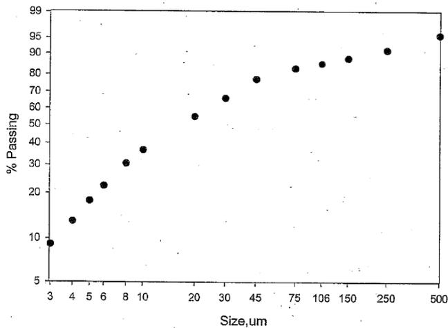
Figure 1. Size distribution of fly ash from Hazelwood power station (Sigma 2003)
