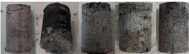
**Figure 8. Five specimens taken before commencing testing retrieved from 6 m to 6.45 m depth tubes.**
