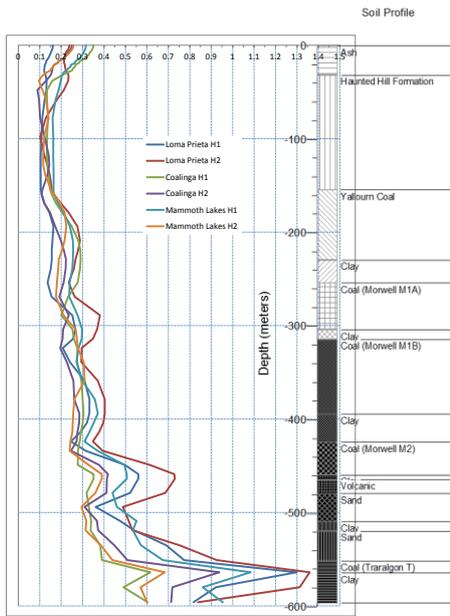
**Figure 6** Peak Ground Acceleration (PGA) through soil profile of HAP4A
