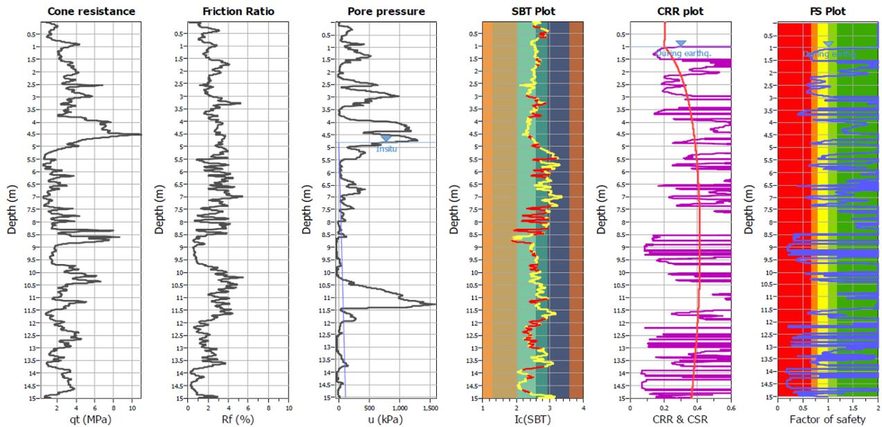
**Figure 7.** Factor of safety against liquefaction for a CPT probe on the crest of ash embankment in HAP4A. (0-4m: Ash Embankment, 4-15 Ash deposits in HAP4)
