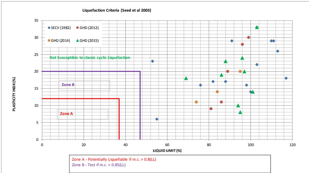
**Figure 3. Results of liquefaction susceptibility based on Seed et al (2003)**
