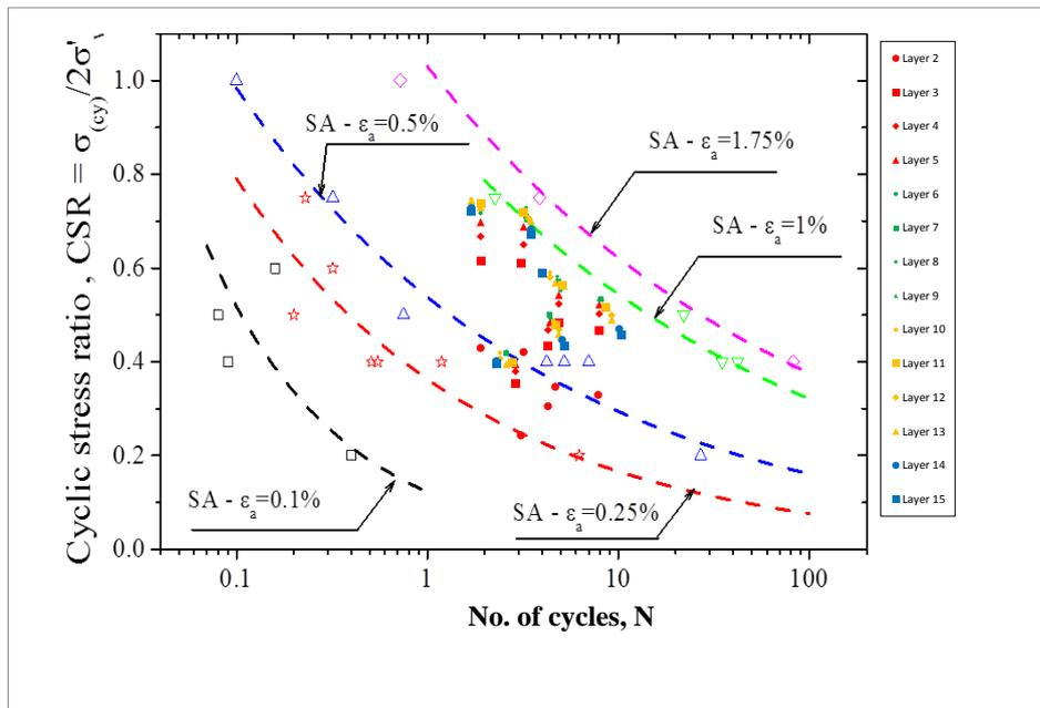
Figure 9 Results of triggering of liquefaction of impounded brown coal ash in HAP4A for MCE events (GHD 2015)
