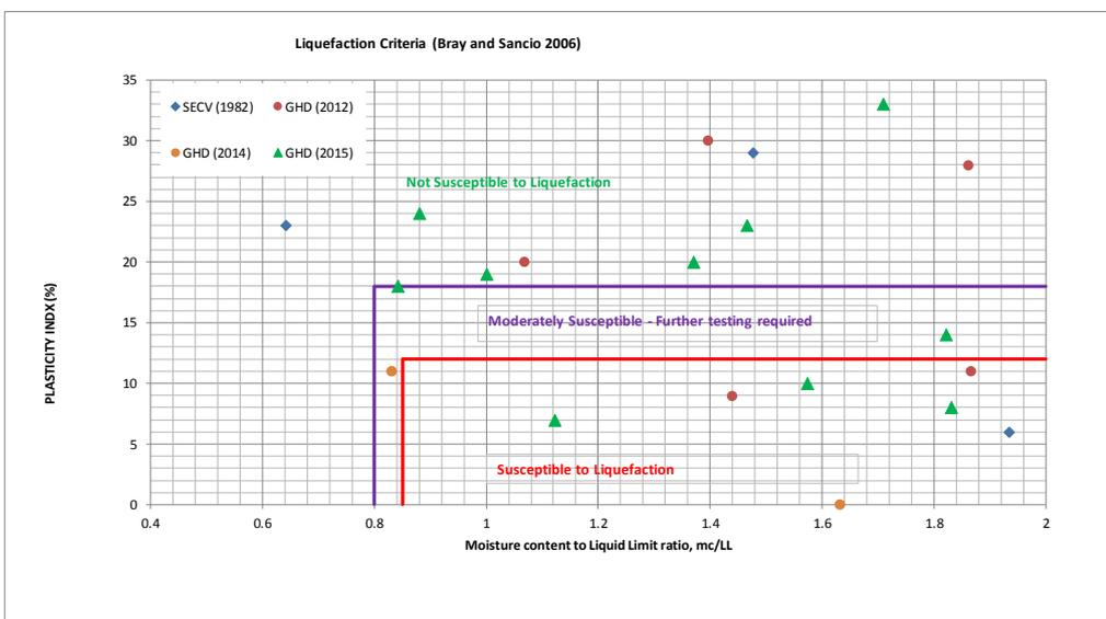
**Figure 4. Results of liquefaction susceptibility based on Bray and Sancio (2006)**
