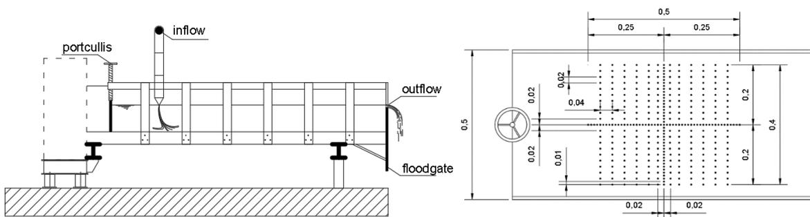
**Fig. 1 Experimental setup and test area with indication of the tap positioning**
