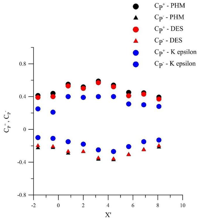
**Fig. 5 Experimental bottom fluctuating pressure parameters  $c_p^\pm$**
