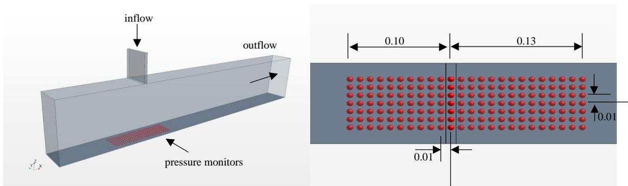
**Fig 2 CFD model setup and test area with indication of the tap positioning**
