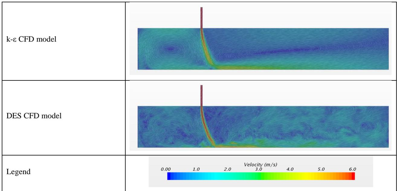
**Fig 3 Comparison of the velocity vectors**
