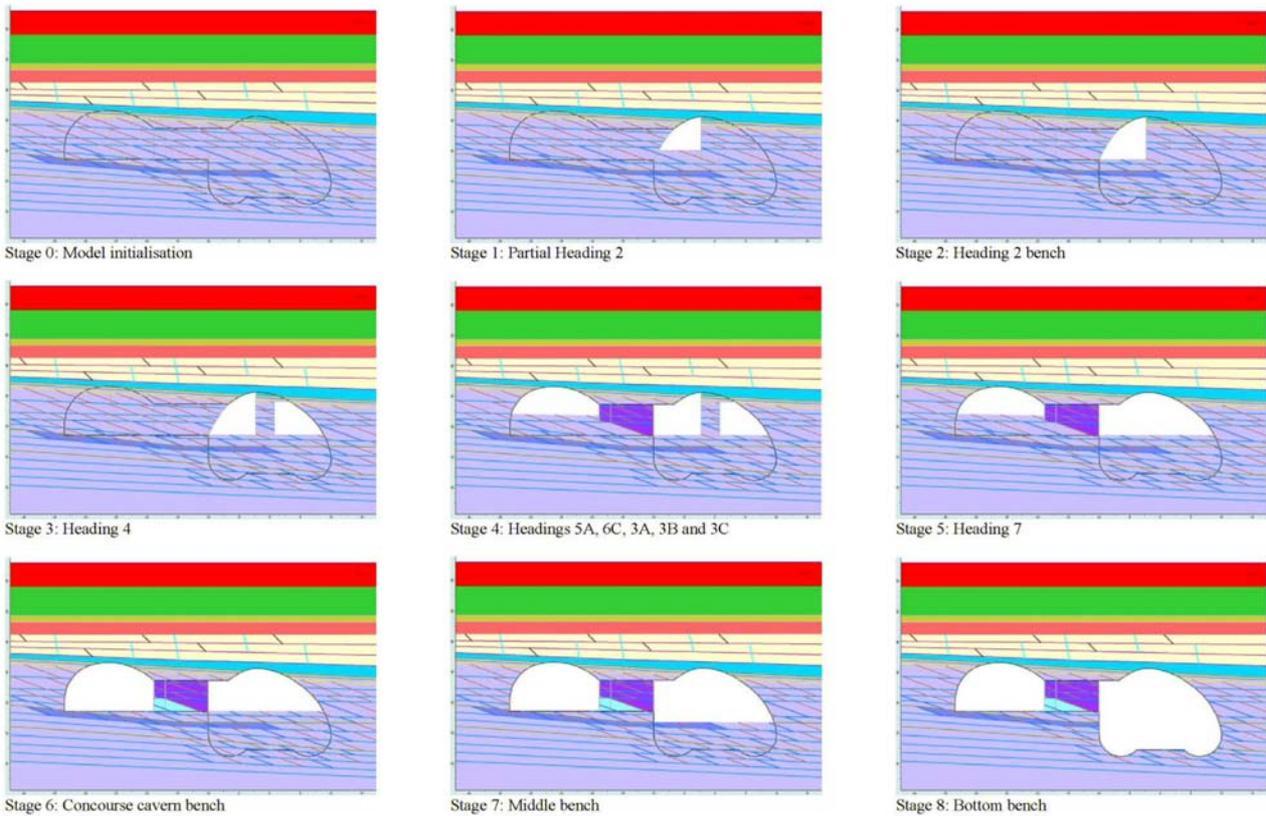
**Figure 4: Back-analysed Construction Stages**
