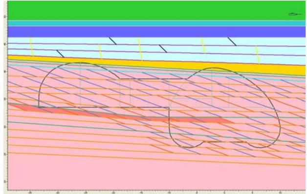
**Figure 3: Back-analysis Finite Element Model**
