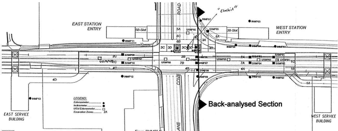
**Figure 1: General Layout of Some of Key Instruments Installed at Macquarie Park Station**
