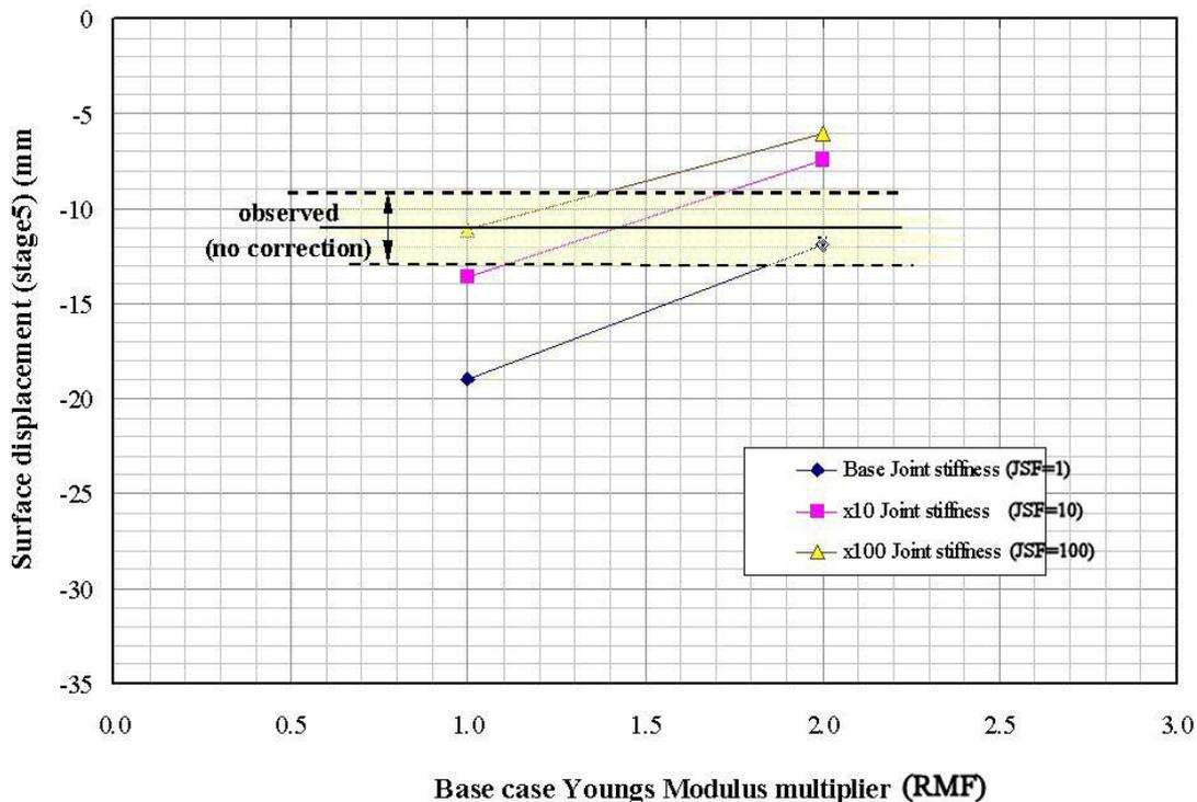
**Figure 5: Plot of Calculated and Measured Ground Surface Displacements with Various Combinations of Rock Mass and Joint Stiffness Parameters**
