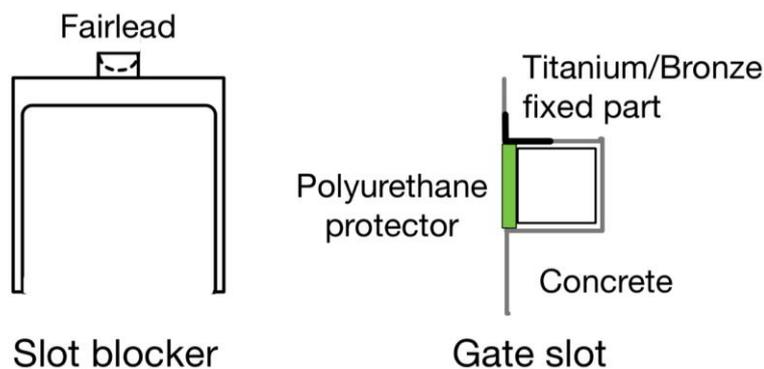
**Figure 5 Slot blocker**
