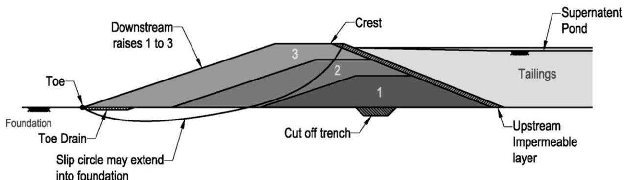
**Figure 5 Typical slip circle location within a downstream raise dam**
