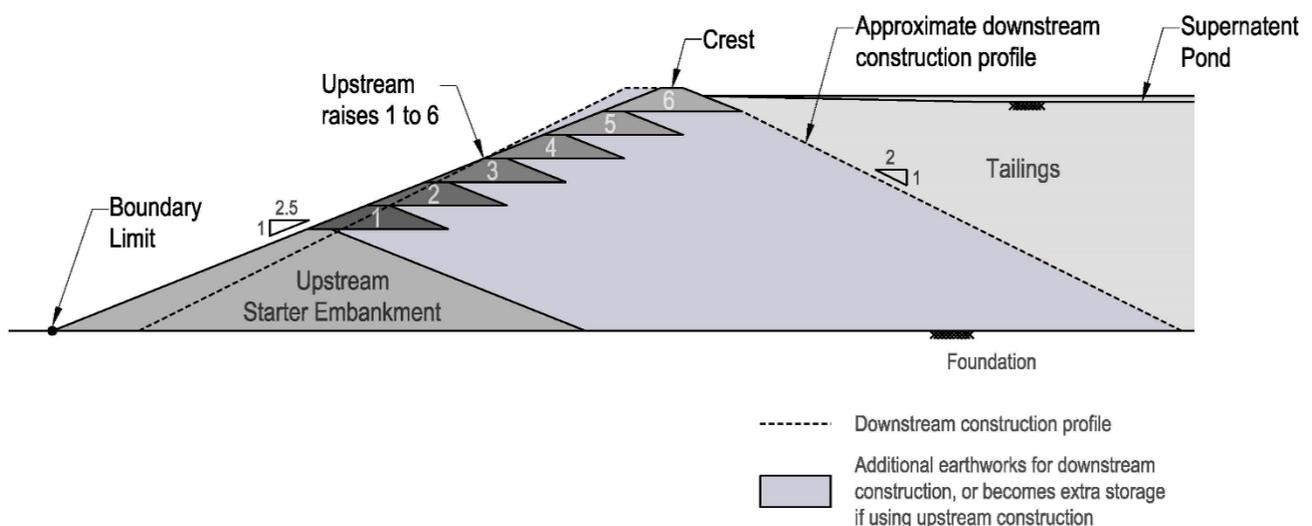
**Figure 3 Increased storage volume with upstream construction (u/s section compared to d/s section)**
