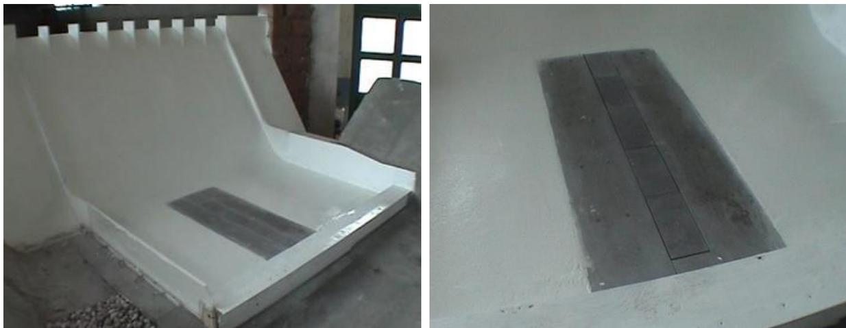
**Figure 4: View of the experimental installation (left) and the test frame within the stilling basin (right)**
