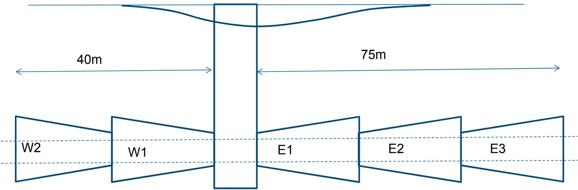
Re-mining using AGF to form 1.5m ice-walls around tunnel
