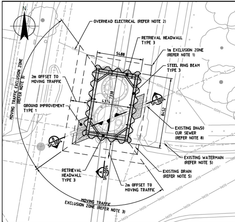
**Figure 4 Woollongabba Trunk Sewer Upgrade Sheet Pile Shaft General Arrangement**
