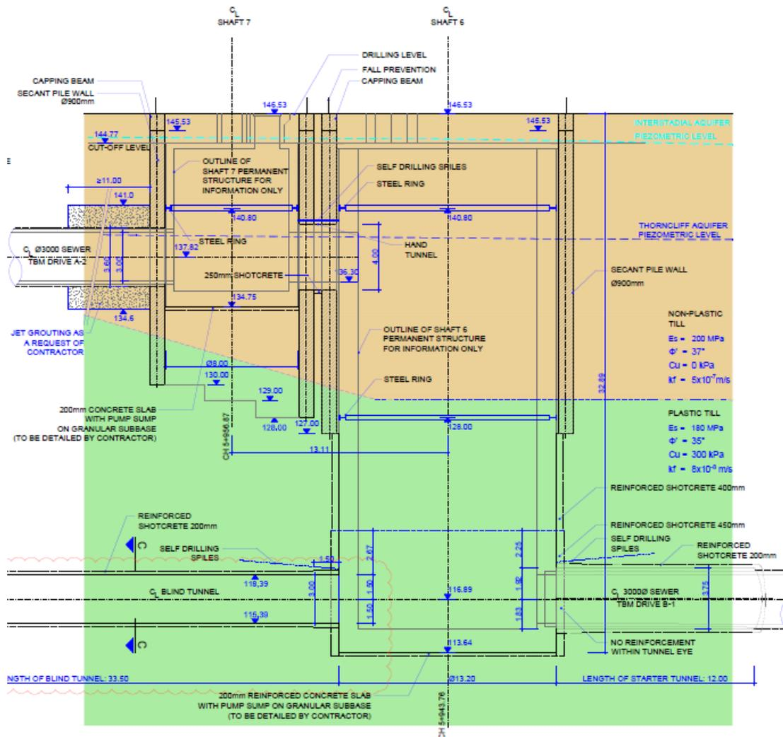
**Figure 2 Southeast Collector Shafts No. 6/No. 7 Secant Pile Shaft Design**
