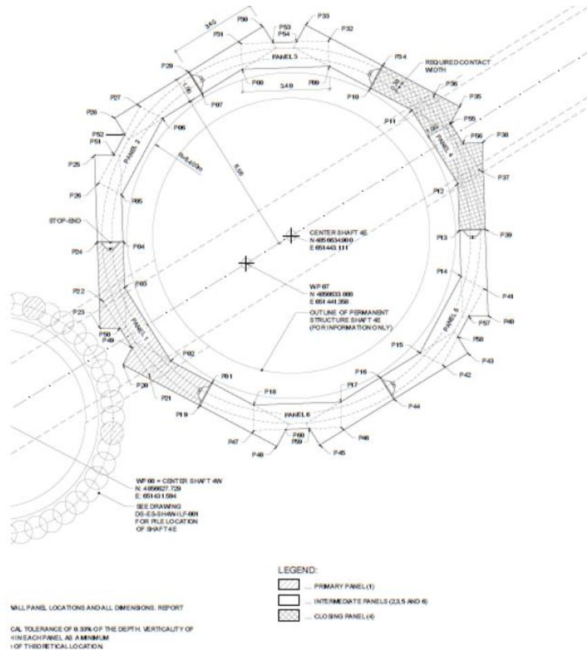
**Figure 6 Southeast Collector Shaft No. 4 General Arrangement**
