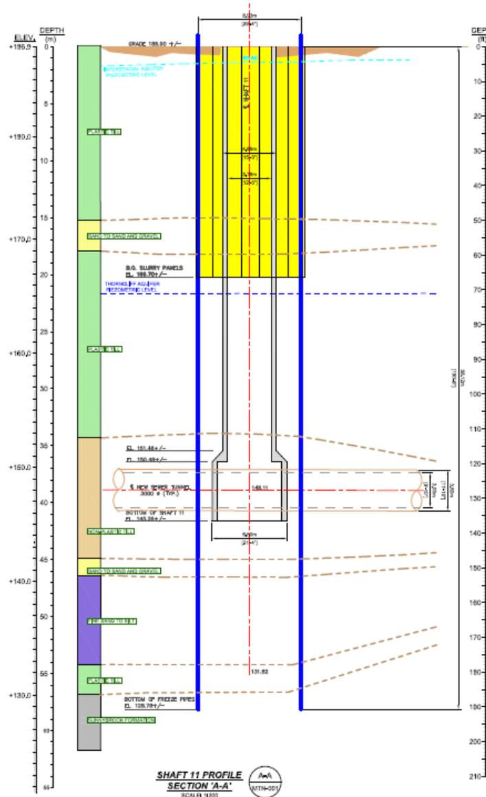
**Figure 8 Southeast Collector Shaft No. 11 Ground Freezing Design**
