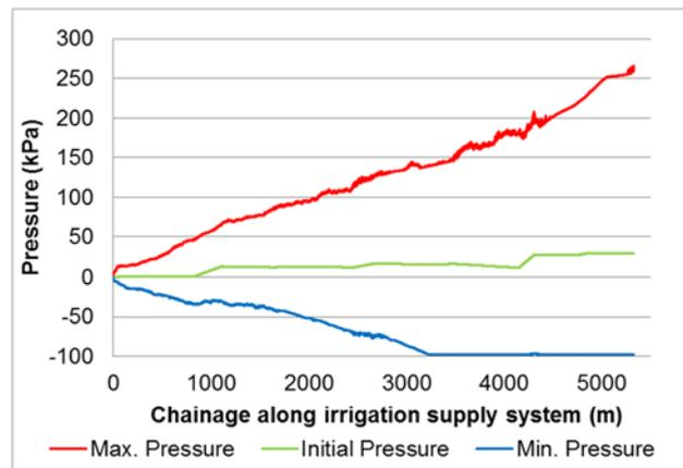
Figure 2: Example of pressure envelope following valve closure.
