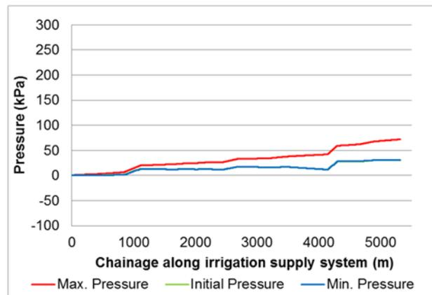
*Figure 3: Example of pressure envelope following valve closure, with inclusion of surge towers.*
