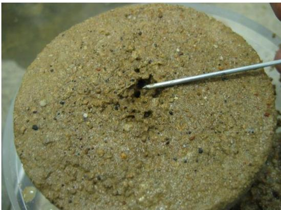
Base of clay core after test
