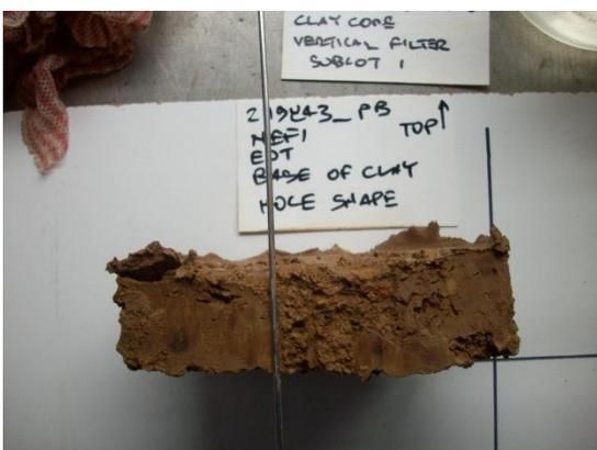
Eroded hole after test
