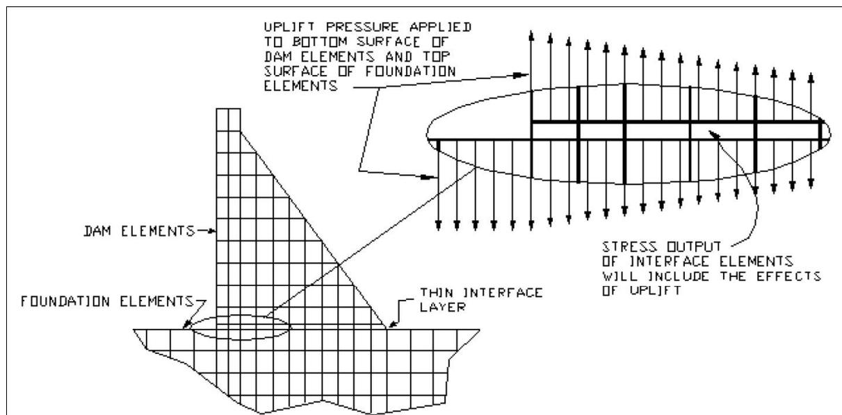
**Figure 2. Application of uplift in a FE model of a concrete dam (from FERC,2002).**
