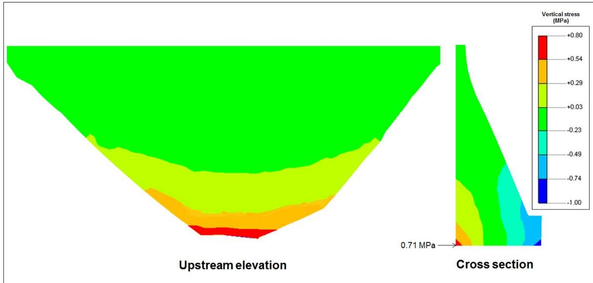
**Figure 7. Resulting effective stresses (uplift and pore pressure combined with static loads)**
