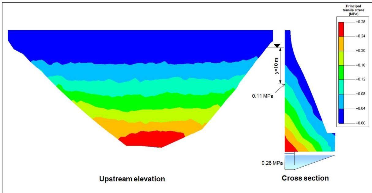
**Figure 6. Principal tensile stresses (uplift and pore pressure loading case only)**
