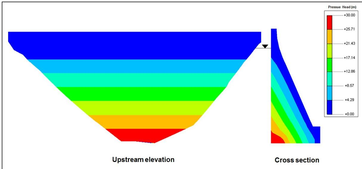
**Figure 5. Resulting pressure heads from prescribed uplift and pore pressures**
