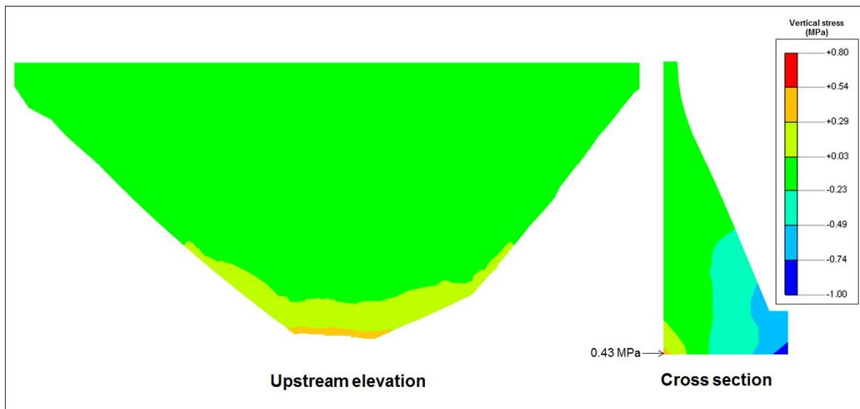
**Figure 8. Resulting total stresses (uplift and pore pressure neglected)**
