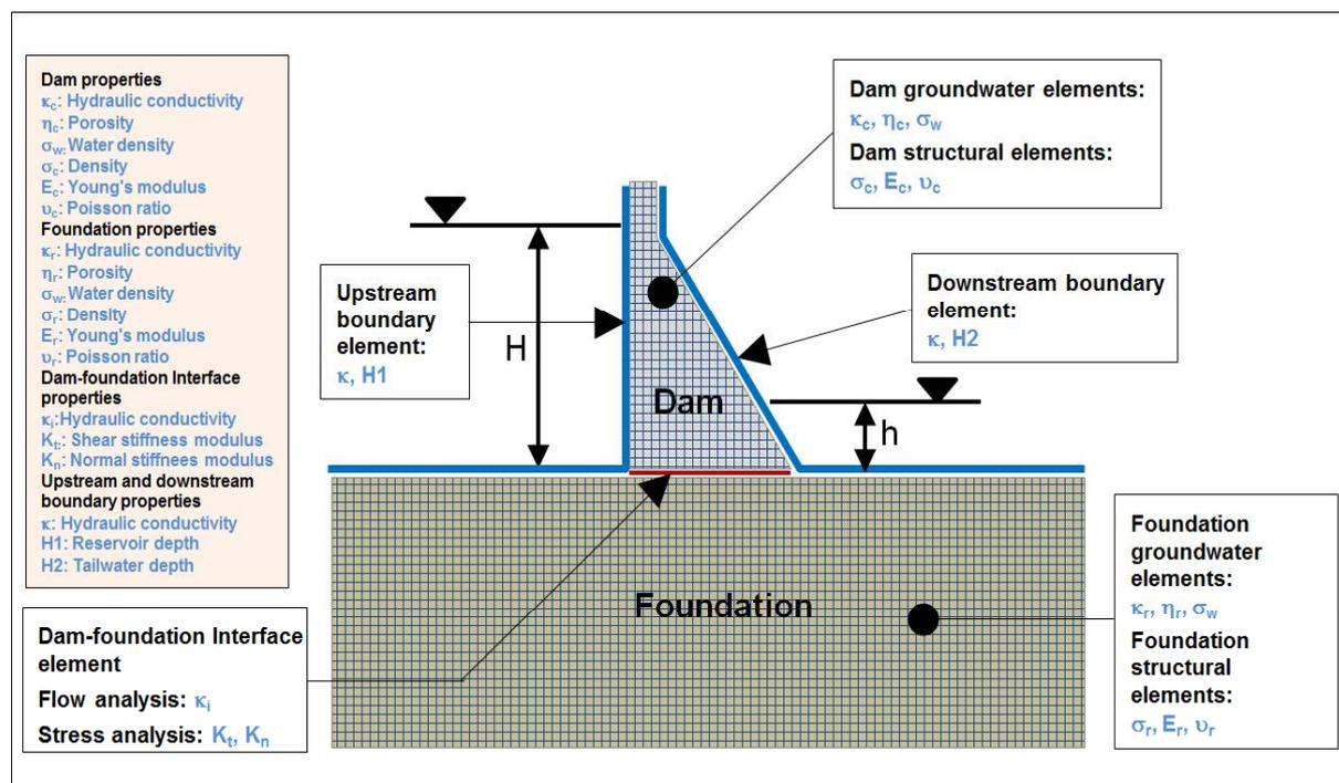
Figure 3. Schematic FE model for coupled steady-state flow and stress analyses
