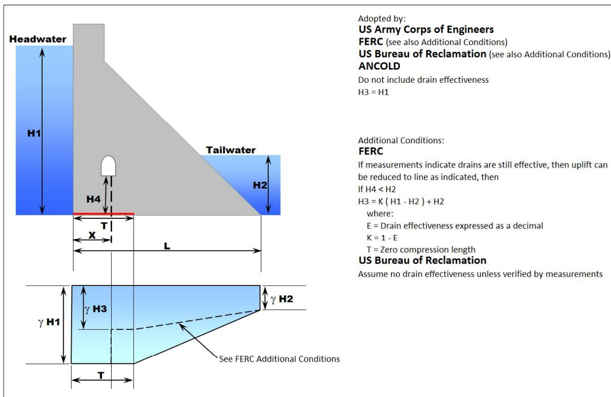
**Figure 1. Uplift formulation for cracked base beyond the drainage line (gallery below tailwater)**
