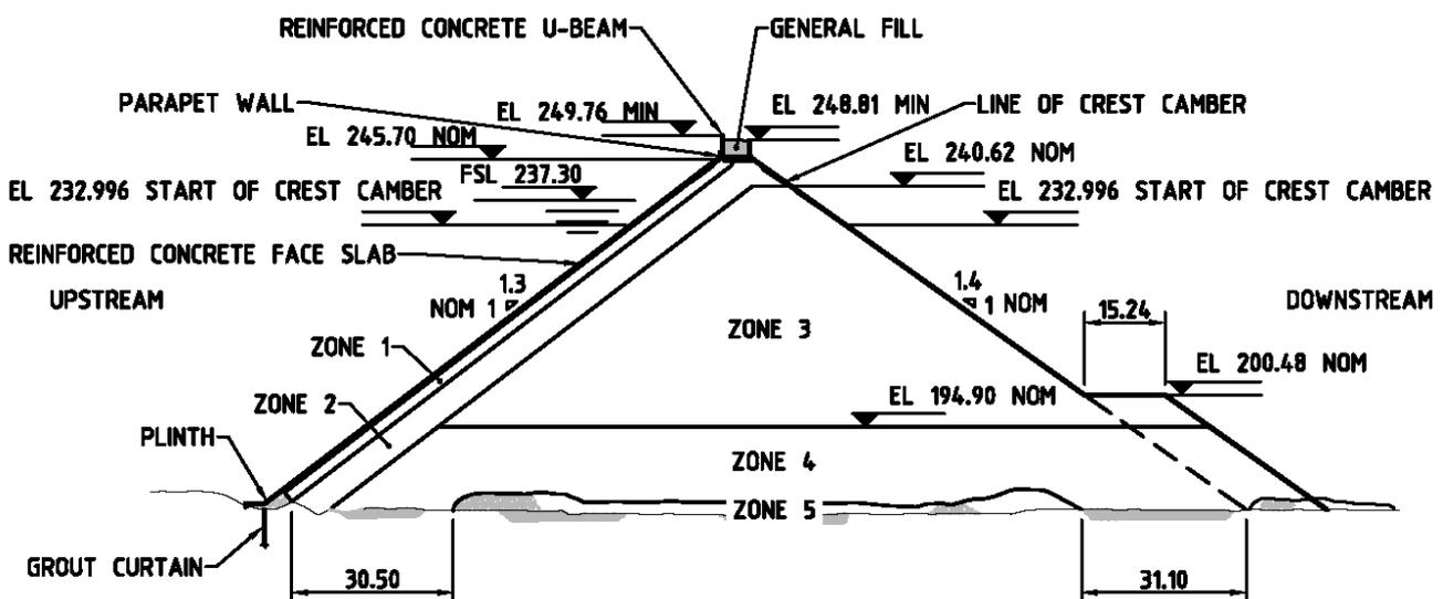
Figure 1 – Typical cross section of the original embankment showing zones (includes 1983 raising)
