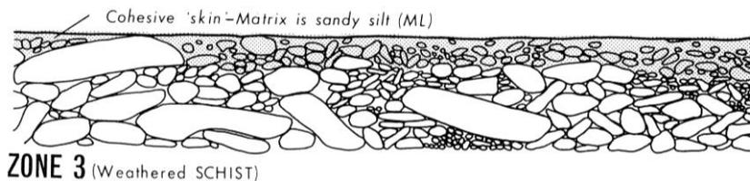
Figure 2 – Illustration of the breaking down of rockfill material during placement (reproduced from Trudinger 1972)
