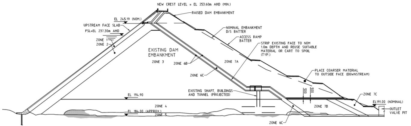
**Figure 4 – Typical cross section of the upgraded embankment**
