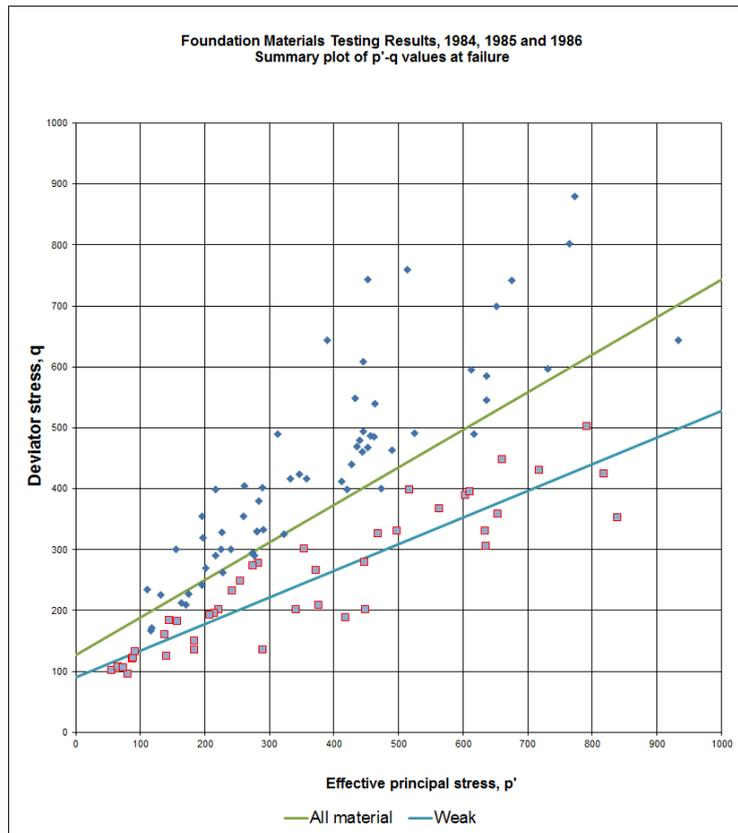
**Figure 4 p'-q lines of best fit**
