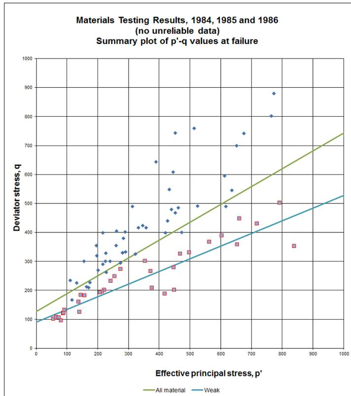
**Figure 7 p'-q plot for all foundation data with possible unreliable data removed**
