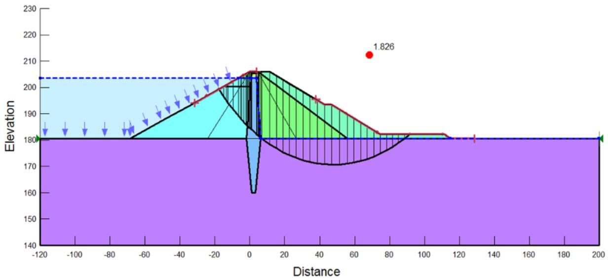
Figure 5 Critical failure slope for "All Data" Foundation
