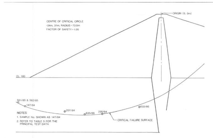
**Figure 1 Stability review with failure surface through selected weak points (late 1980s)**
