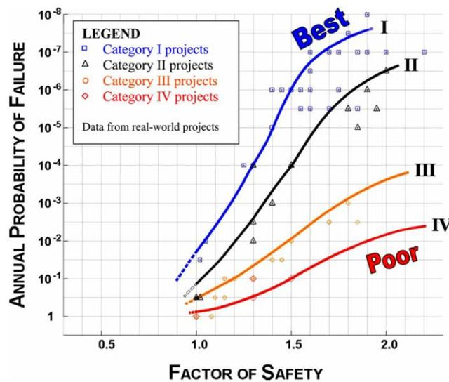
**Figure 8 Factor of Safety versus annual probability of failure (Silva et al., 2008)**
