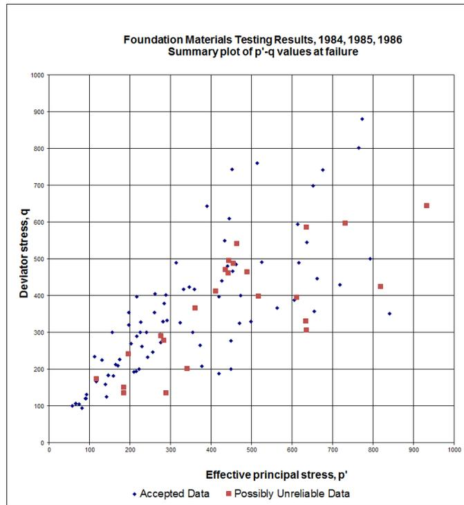
**Figure 3 p'-q plot for all available foundation data**
