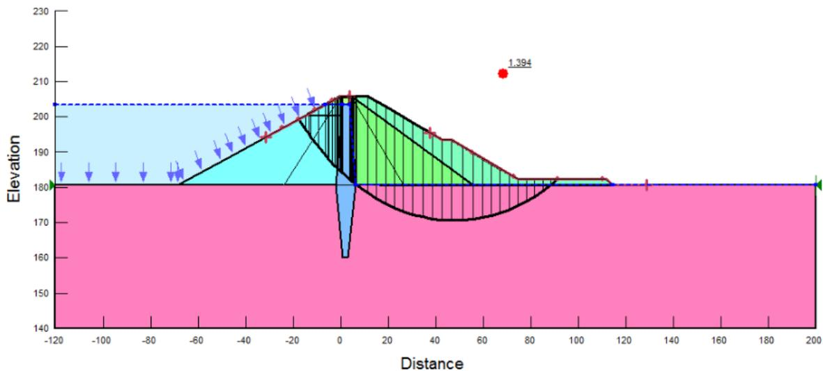
Figure 6 Critical failure slope for "Weak" Foundation
