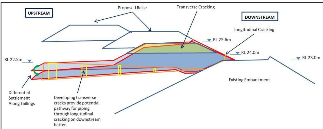
The most significant root causes for the longitudinal cracking were determined by consensus of the participants during discussions in the meeting, as shown on Table 3.
