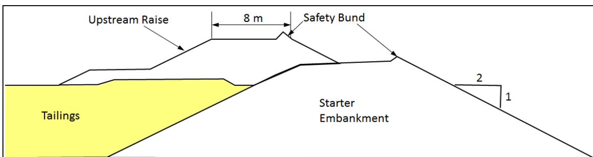
The deposition into the storage facility was by means of spigots spaced at about 25 m centres along the upstream crest. During routine inspections two years after completion of the raise, transverse cracks of up to 30 mm were noted on the crest and longitudinal cracks up to 40 mm width were noted on the downstream slope of the raised embankments, with a typical pattern shown on Figure 4.
