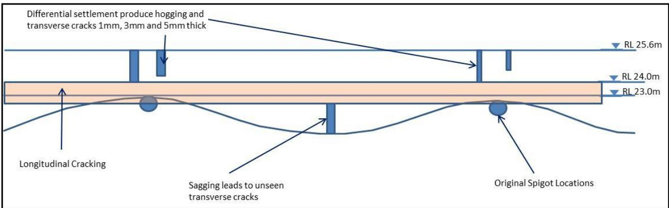
**Longitudinal Cracking Root Cause Analysis results**
