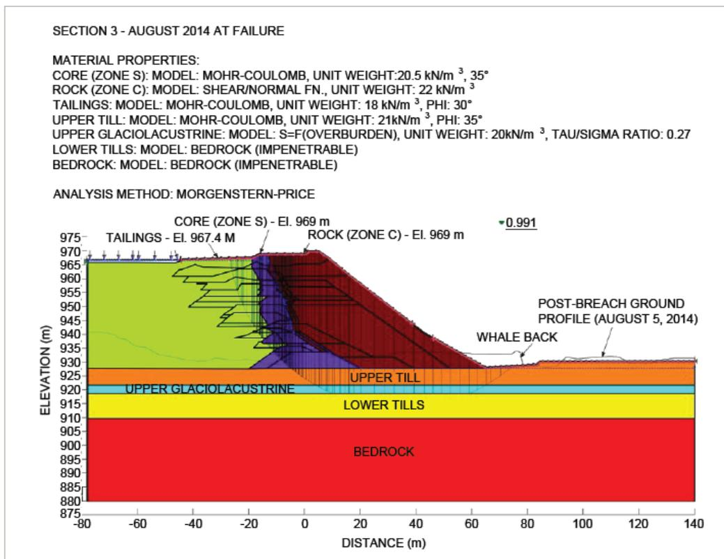
**Figure 2** Calculated failure surface Mt Polley Tailings Dam (reproduced from Panel report)
