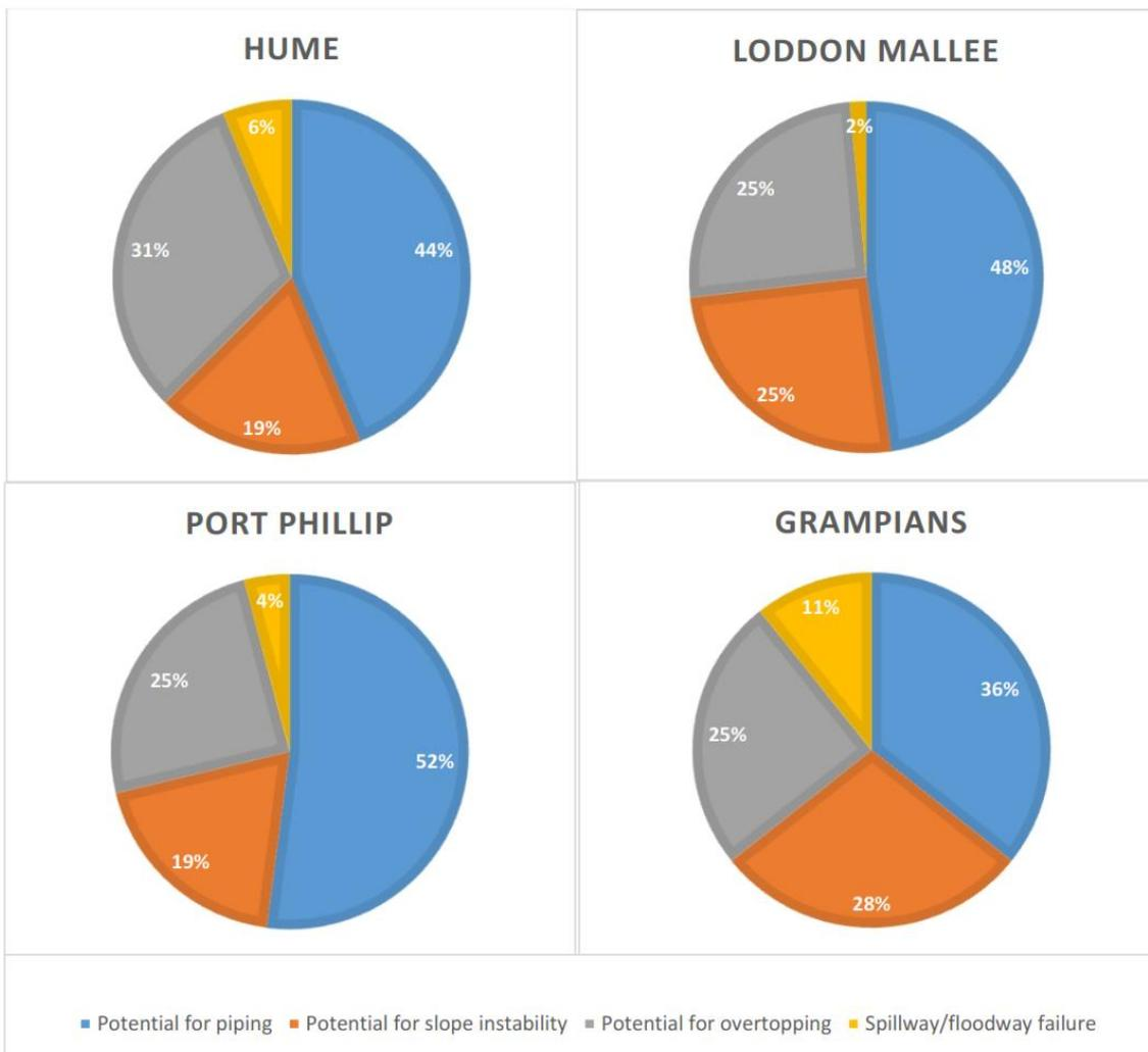
Figure 7: Predominant Failure Modes per Region for Embankment Dams
